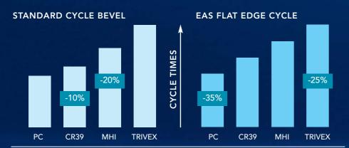
Significant time savings compared with current generation platforms. Average cycle times observed on a range of lenses between -3.00 D and +3.00 D.
